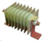
The K-series integrates metal fins into the disc resistor stack to improve forced or free air convection cooling, obtaining a higher average power rating. This technique also reduces cool-down time in crowbar or dump applications when repetitive operations is a requirement.
