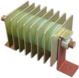
The K-series integrates metal fins into the disc resistor stack to improve forced or free air convection cooling, obtaining a higher average power rating. This technique also reduces cool-down time in crowbar or dump applications when repetitive operations is a requirement.
